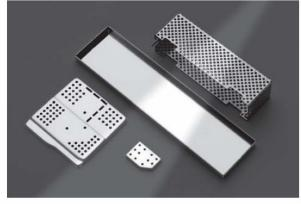
Custom one-piece cans with half-etched bend lines and 'Quiet' construction features offer outstanding attenuation combined with excellent coplanarity for ease of assembly. These can be shipped fully formed or flat pack for self-assembly, either manually or with soft tooling. They can be virtually any size and can incorporate a wide variety of design features to enhance performance and ease of use.
