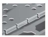
enable vacuum manipulation. In a two-piece can a special land is designed into the can body. It can be easily removed with a simple twist after assembly and before the lid is finally positioned.
